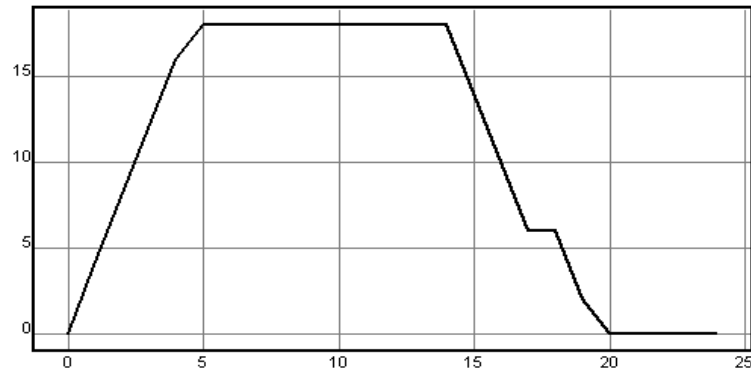
Trapezoidal Position profile. Automatic elimination of round-off errors
